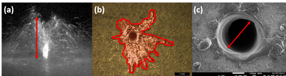
Figure 1.6: (a) Height of the fountain. (b) Recasted material area around the hole. (c) Diameter of the hole.
