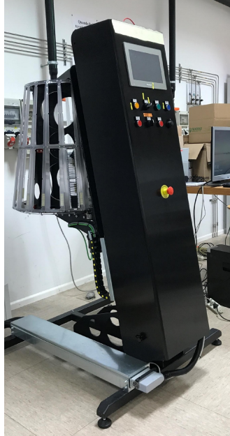
Figure 3.5: The HORUS machine. The rotating wheel is visible at the back of the device.
