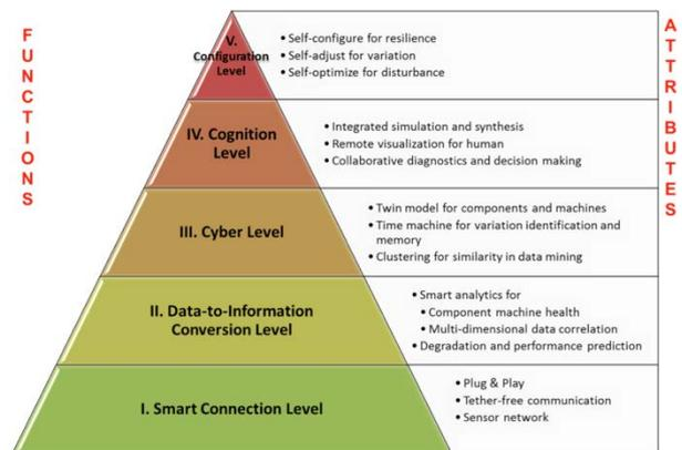
Fig. 6. Cyber-physical systems for manufacturing (source: Wikipedia.com).
