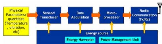
Fig.1. A typical WSN architecture.
