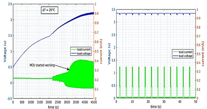
Fig 4. Current and voltage during charging phase (a) and after supercap was fully charged (b).
